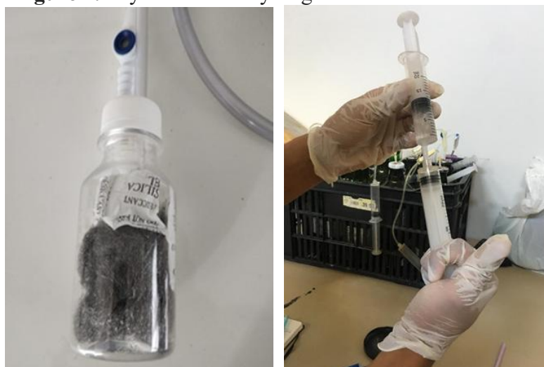
Figure 4. Dry reaction of hydrogen sulfide with iron oxide
