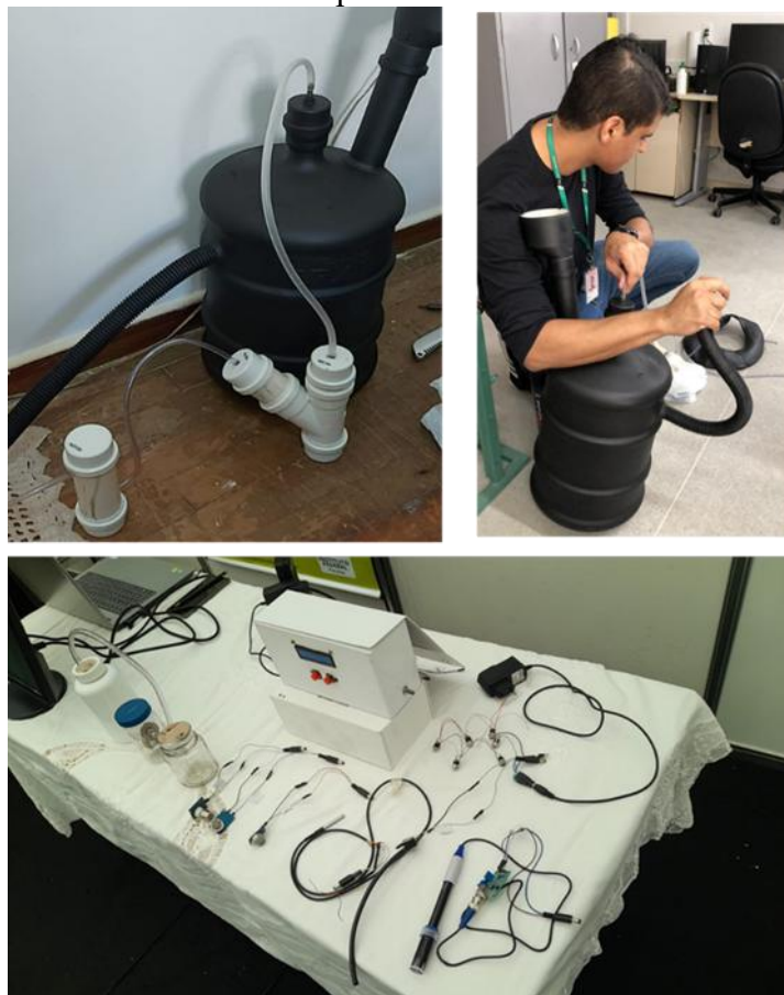
Figure 7. Flumen Gas Project – gas production tests and sensor system used on the Arduino 1 platform.
