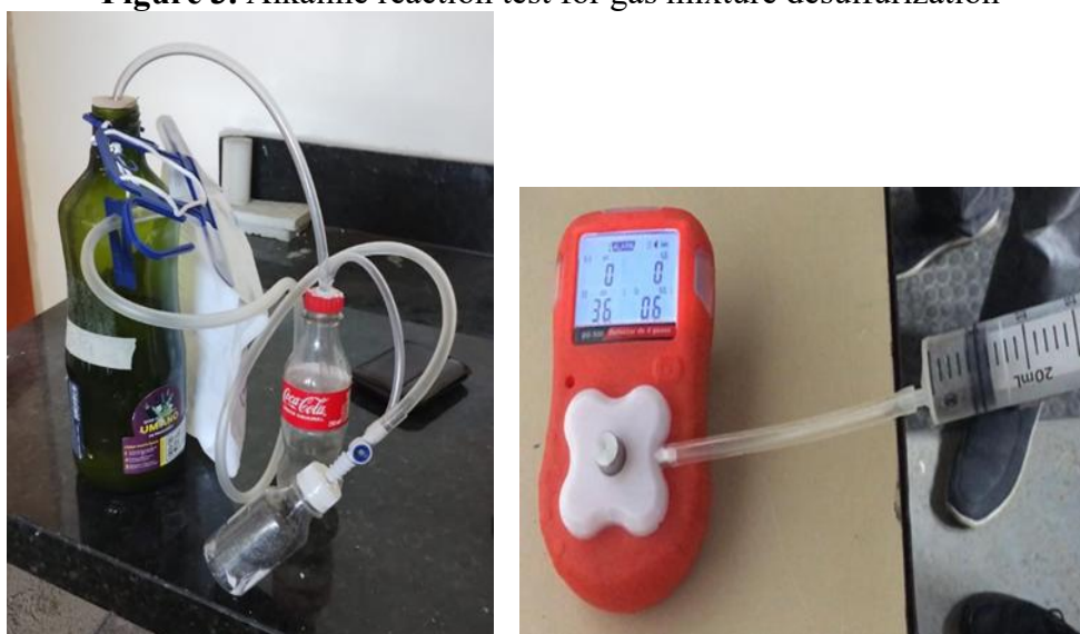
Figure 3. Alkaline reaction test for gas mixture desulfurization
